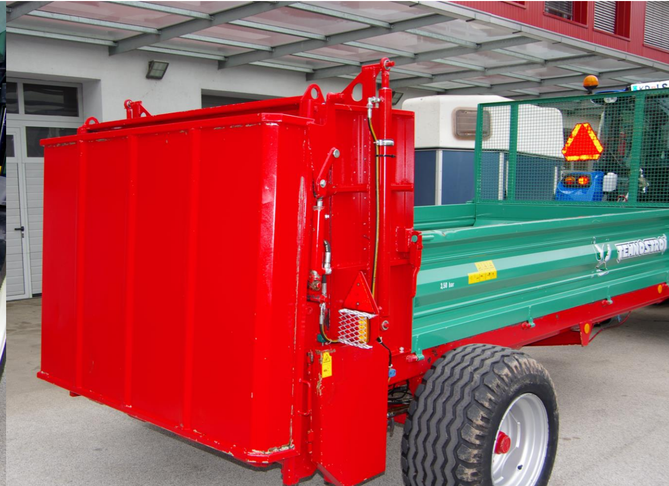
Hydraulic closing and dosing door in front of the spreading device
