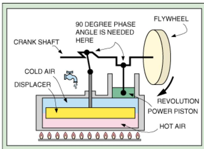
They are used only in some very specialized applications, like in submarines or auxiliary power generators for yachts, where quiet operation is important. Although there hasn't been a successful mass-market application for the Stirling engine, some very high-power inventors are working on it.
